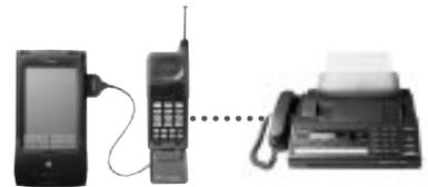
The Newton communications architecture enables users to take advantage of cellular devices to connect to e-mail systems, dial-in services, and fax machines.
